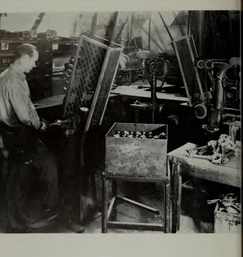
The cap is replaced on the rod using the original bolts and nuts, the removal of which was described in Picture 5. A power driven socket wrench is used in performing this operation.
